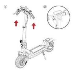
$3.\ \ensuremath{\boxdot{\text{l}}}\xspace$  Cut the tapes on the handlebars and lift up the handlebars
