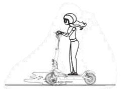
Do not ride in a ponding that is higher than 20mm.
