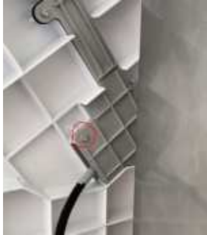
Figure 7: Screw that needs to be removed inside of bezel
