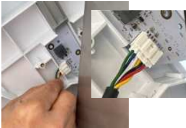
Figure 8: LED Cable Connector with Tab
