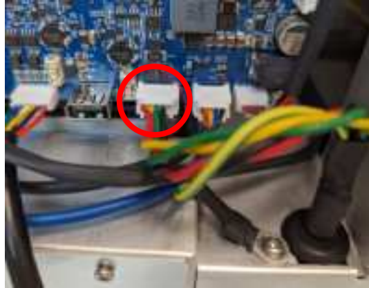
Figure 20: Four-Wire Connector Placement on the Control Board
