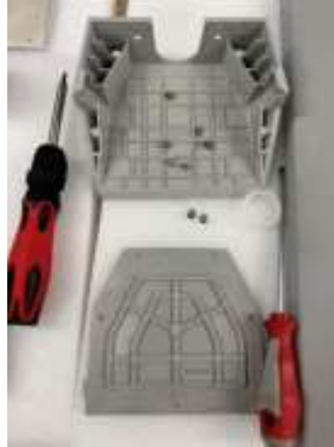
Figure 25: Transition cover (top) & sealing cover (bottom)
