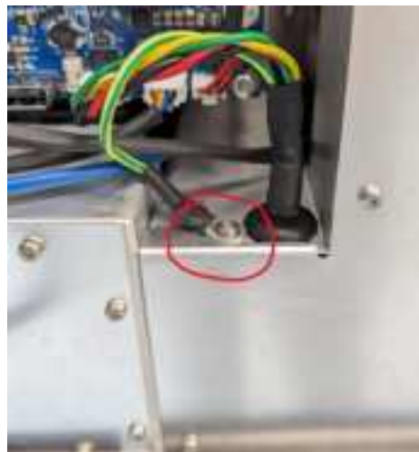
Figure 21: Ground Screw where Yellow/Green Stripe Cable Connects
