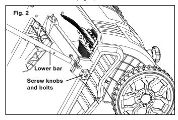
Secure the handle to the lower bar using two sets of screw knobs and bolts (Fig. 3).
