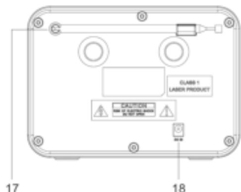
17 Telescope antenna
