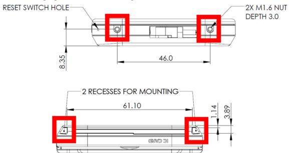
• Likewise, the VP3350 has slots on the back for alignment, shown below:
