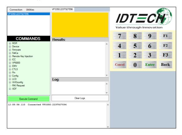
The Universal SDK Demo app displays VP3350's available commands in a command tree, as shown above. Single-click on a command to populate the center panel of the window with optional settings relevant to the command (for example, "Amount" and "Start EMV Additional Tags" above). In some cases, text fields appear, allowing users to enter custom values.
