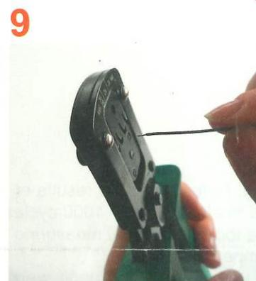
9 Insert the cable until insulation
