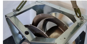
Fitting lifting lugs in the positions provided
