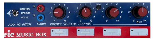
Only one "preset voltage source" can be selected at a time as indicated by the LEDs. The knob above each pad sets the output CV from 0-10v. The corresponding voltage will appear at the blue "output" banana when that knob/source is selected.
