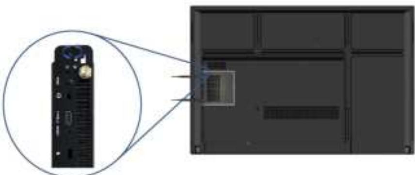
**Step 5:** Press the small Power Button on the back of the OPS to power it on. It can also be powered on from the 'Source' option in your OneScreen Panel.
