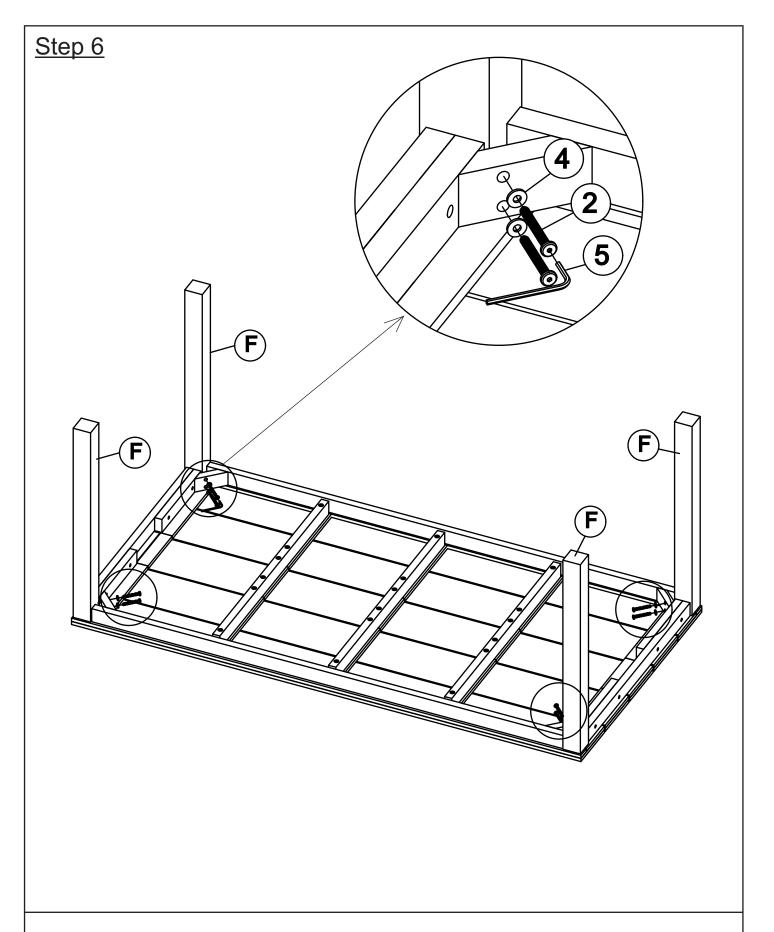
Attach the Leg (F) onto the Table Top using Bolts 2 , Washers 4 , and the Allen Wrench 5
