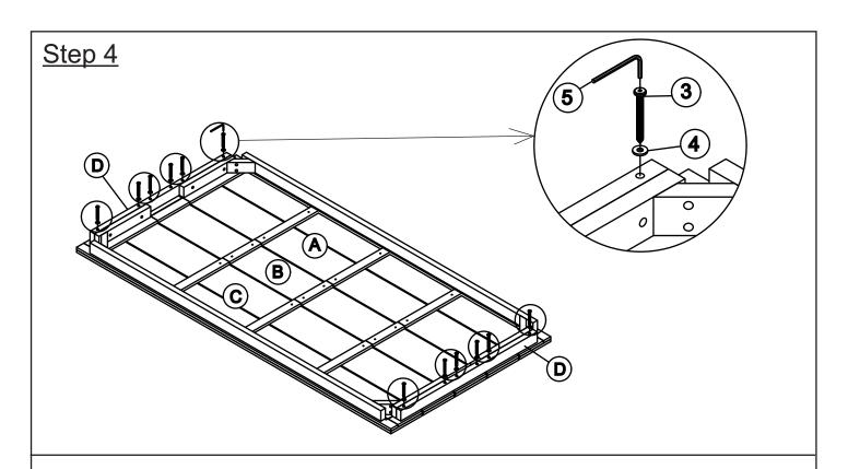
Secure a Side Support Bar (D) to the apron of the Table Top using Screws 3, Washers 4 and the Allen Wrench 5 as shown in the picture above. Repeat the same process with the remaining Support Bar (D) **DO NOT fully tighten the Screws**.
