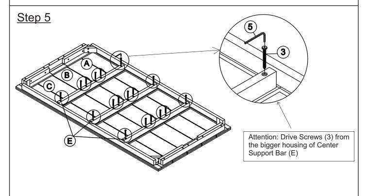
Attach the Center Support Bar (E) onto the Table Top using Screws and the Allen Wrench (5)
