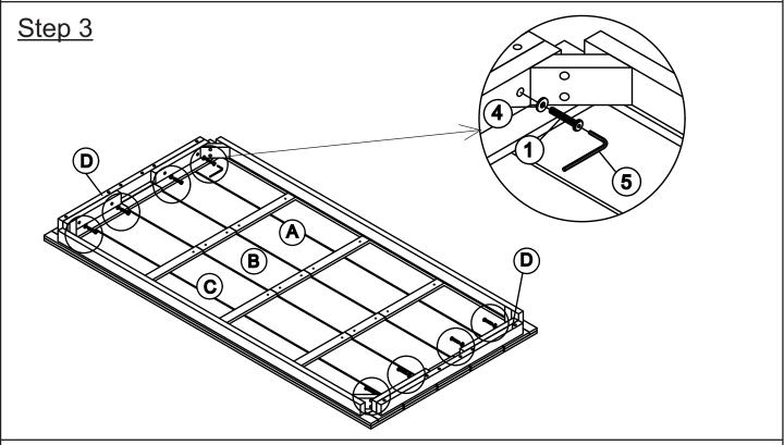
Attach the Side Support Bar (D) into the shorter side of the Table Top using Bolts 1, Washer 4 and Allen Wrench 5 as shown in the picture above. Repeat the same process with the remaining Side Support Bar (D)
