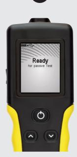
Press the Test key — the screen will display "Please Wait" then "Ready for passive Test".
