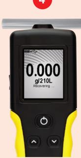
A screen with the numerical BrAC of "0.000g/210L" indicates that alcohol is not present.
