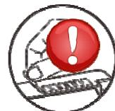
When powering on for the first time, open the battery cover, remove the sticker from the top of the battery, and insert the lithium battery.
