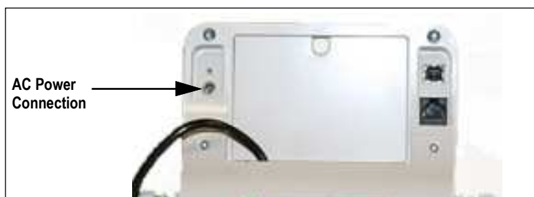
Figure 2-6. Power Connection Site
