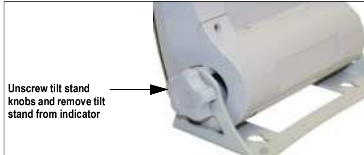
Figure 2-2. Remove Tilt Stand
