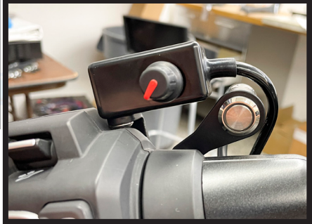
Dimmer and switch mounting location
