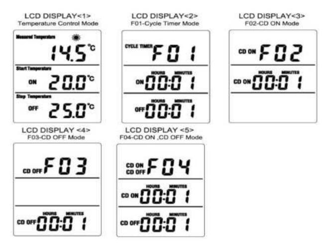
F01 Cyclic Timing Mode: Cycle by start time (ON) and stop time (OFF).
