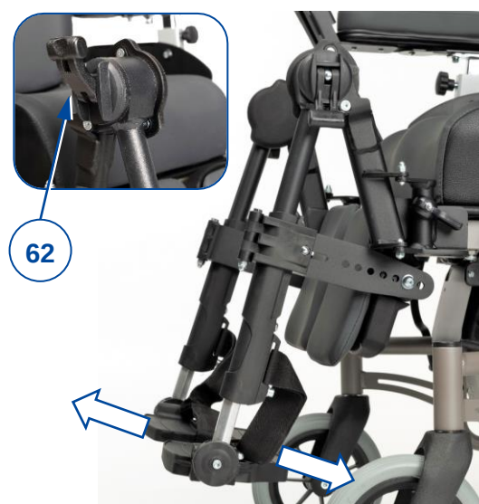
Figure 9 Adjusting footrest angle
