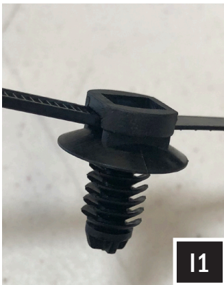
I1. Place zip-tie through zip-tie post. Press zip-tie post into the zip-tie post holes that follow down the center of the vehicle. Starting from the rear of the vehicle, zip-tie the speaker cable to the vehicle and zip-tie post that were pressed in down the center of the vehicle in the previous step. Coil and zip-tie any slack in the harness towards the front of the vehicle.
