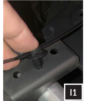
I1. Place zip-tie through zip-tie post. Press zip-tie post into the zip-tie post holes that follow down the center of the vehicle. Starting from the rear of the vehicle, zip-tie the speaker cable to the vehicle and zip-tie post that were pressed in down the center of the vehicle in the previous step. Coil and zip-tie any slack in the harness towards the front of the vehicle.
