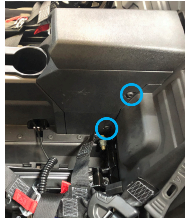
M. Remove the (2) T40 torx screws from both sides of the center console and lift out the rear portion of the center console.
