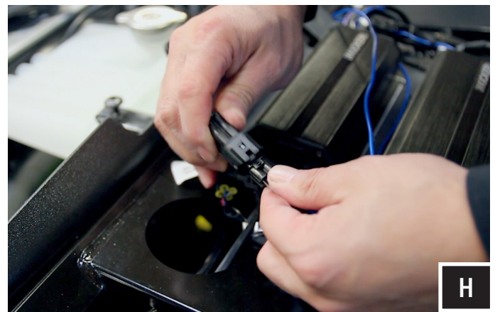
H. Connect the subwoofer cable to the 800.5 amplifier output.
