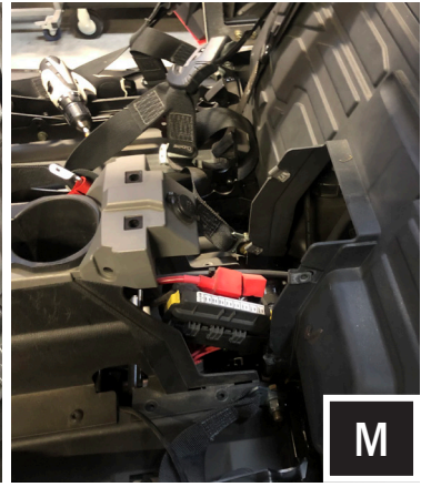
M. Remove the (2) T40 torx screws from both sides of the center console and lift out the rear portion of the center console.
