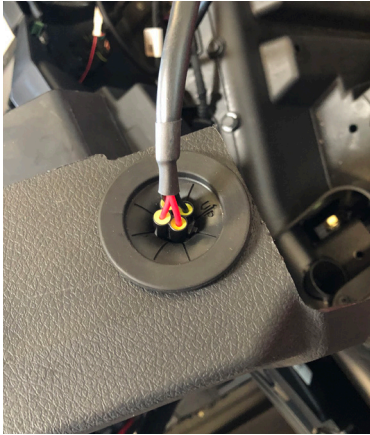
A. Route both of the expansion harnesses down the dash cavity and through the grommet on the front of the passenger console side panel.
