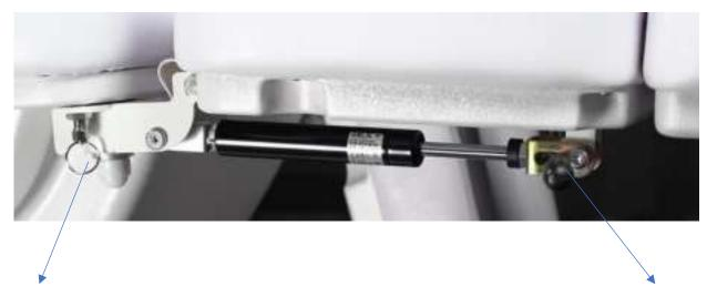
Mechanism for tilting the footrest sideways
