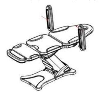
2. Manual control function (lifting height: the bed is 58~ 82 cm from the ground)
