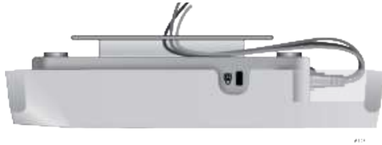
Figure 22. Fitting the Cables in the Cable Hide
