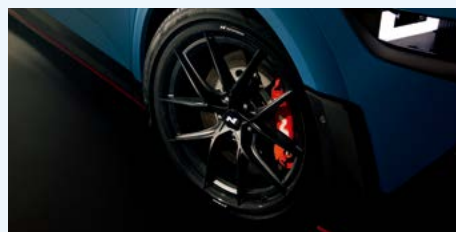
Dymag 21-inch carbon hybrid wheels
