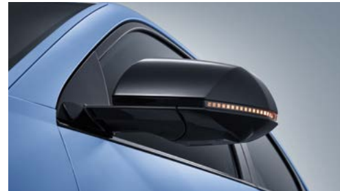
Black outside mirror(heating, power-folding, power adjustment, LED turn signal lamps)
