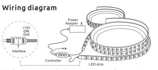
Note: Connect the load wire at first, following by the power wire; Please ensure short circuit can't occur between connecting wire before you turn on the power.
