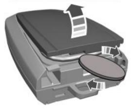
Twist a thin coin under the tab hidden behind the key blade head to remove the battery cover.
