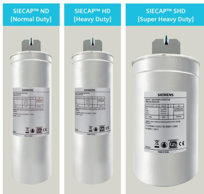
SIECAP™ range of capacitor is based on MPP technology [Metalized of Zinc Al alloy over Polypropylene dielectric] of film making with an impregnation of semi-dry biodegradable soft resin.
