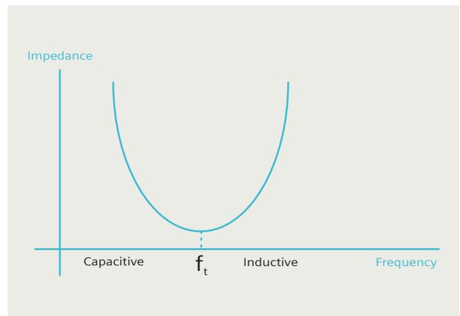
This combination of detuned LC filter will act capacitive for frequency below  $f_t$  and inductive for frequency above  $f_t$ . Thus for base frequency of 50 or 60Hz this detune filter will act as capacitive and improves the power factor. This LC detuned filter is selected such that the tuning frequency is much less than the dominant harmonic frequency. Thus harmonics always see higher impedance and the condition of resonance with feeding transformer is avoided.
