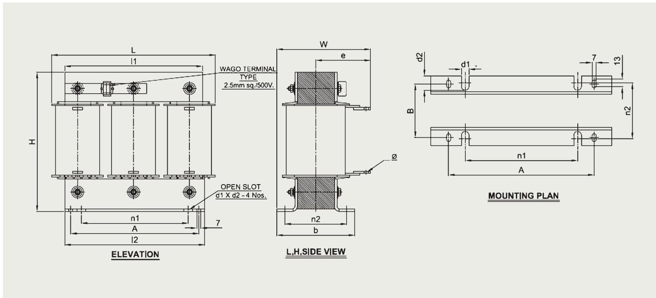
**14% Cu detuned reactor (all dimensions in mm)**
