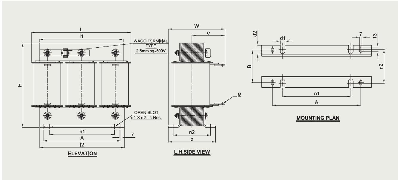
**5.67% Cu detuned reactor** (all dimensions in mm)
