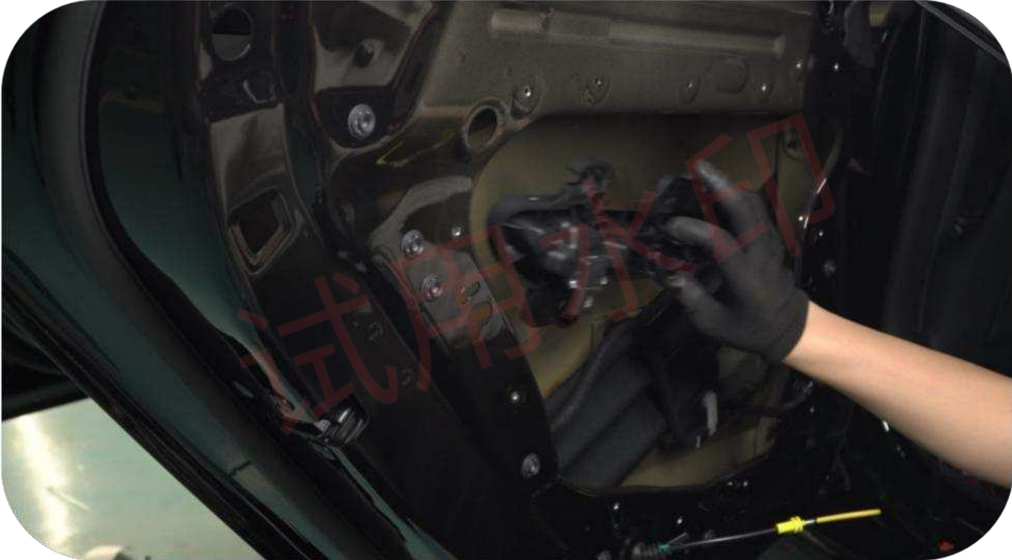
42. Take out the original handlebar
