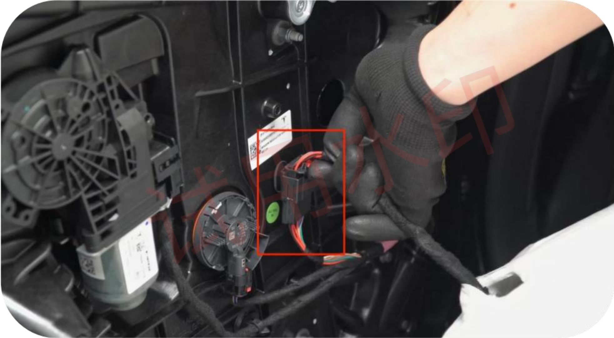
33. Pull out the main harness plug of the door panel
