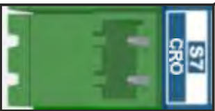
Example of the position of (Hydraulic crossover) CRO on the main PCB UniDrive.
