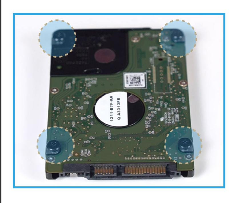
ii. Install the 2.5" HDD screws on your SSD screw holes.
