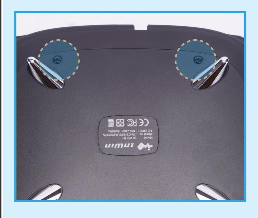
i. Release the two screws and remove the bottom cover.
