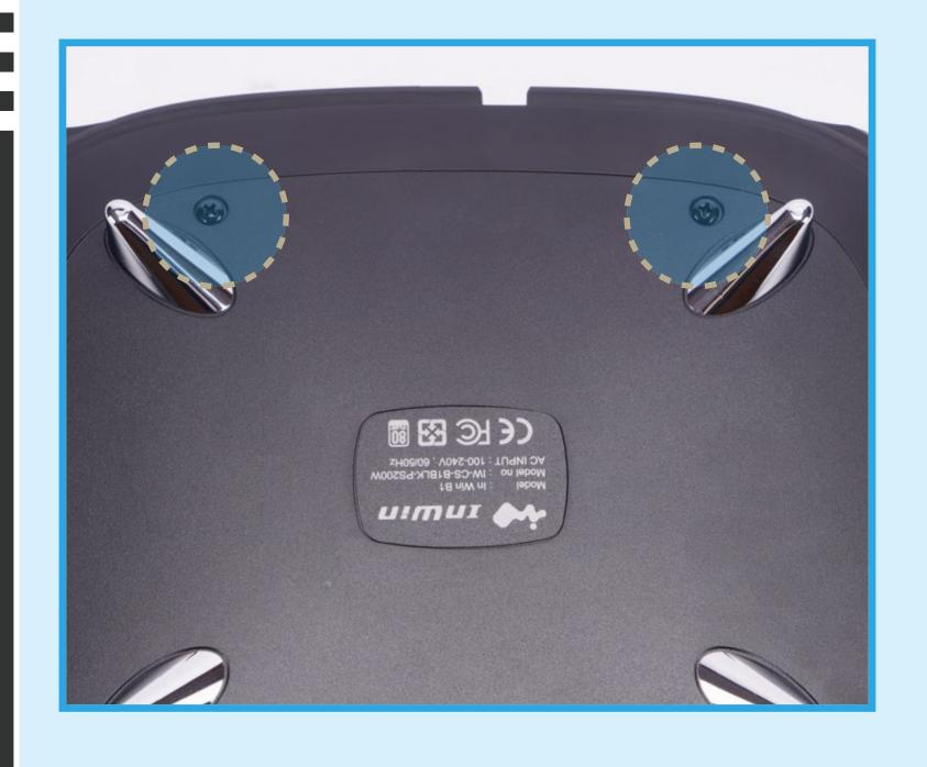
i. Release the two screws and remove the bottom cover.
