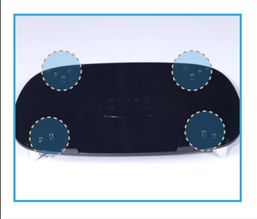
ii. Release the screws of the foot-stand and detach the foot-stand.
