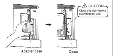
Turn on the power supply, wait until the initialization is completed (the lower panel is in the closed position). Open the door, remove the WLAN adapter and check that the [POWER] lamp for the product lights. After checking, return the WLAN adapter into the unit and close the door.
