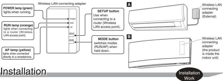
Attach the Wireless LAN connecting adapter to indoor unit.
