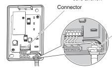
Ensure that the connector on the connecting cord is firmly inserted all the way.
