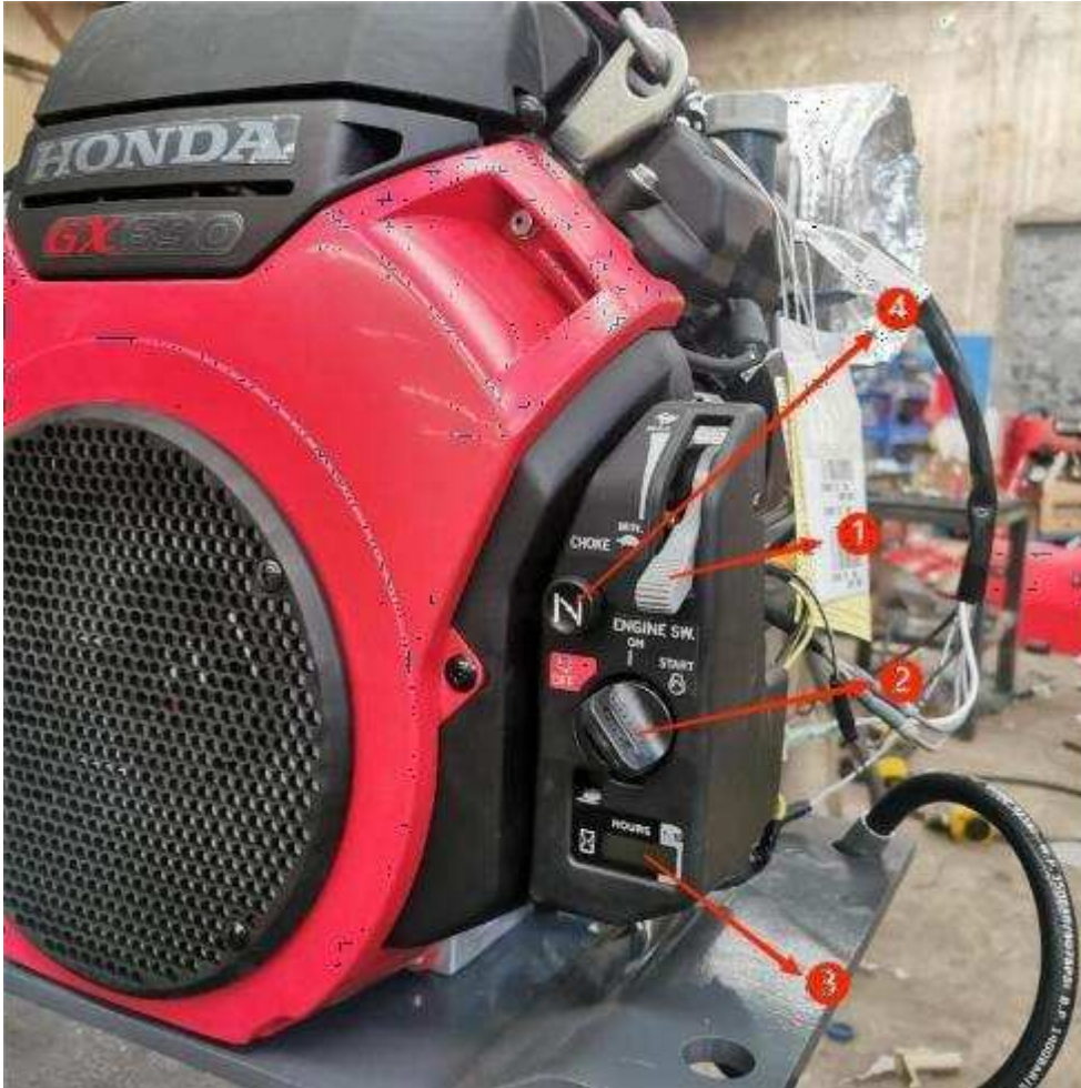
1. Hand Throttle 2. Key Switch 3. Engine Hour Meter 4. Engine Airflow Regulator
