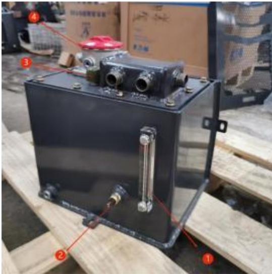
1.Liquid level meter 2.Oil temperature sensor 3.Respirator 4.Oil return cartridge
