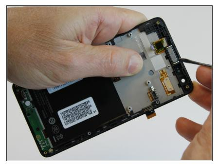
Using the nylon or metal spudger, gently pry the front speaker from the screen assembly.
