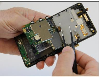
• Using one prong of the tweezers, lift and pry back the metal clip positioned over the front proximity sensor ribbon connector.
