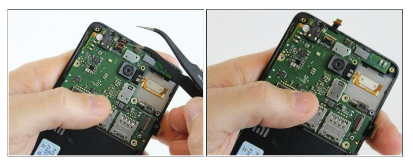
Using one prong of the tweezers, pry the ribbon clip away from the motherboard.
