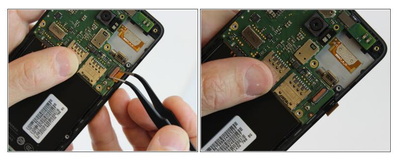
Using one prong of the tweezers, pry back the brown clip located on top of the LCD ribbon connector.
