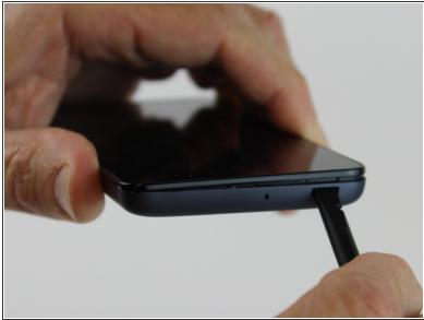
• Use the flat end of the spudger to remove the back panel from the mid-frame and front body.
