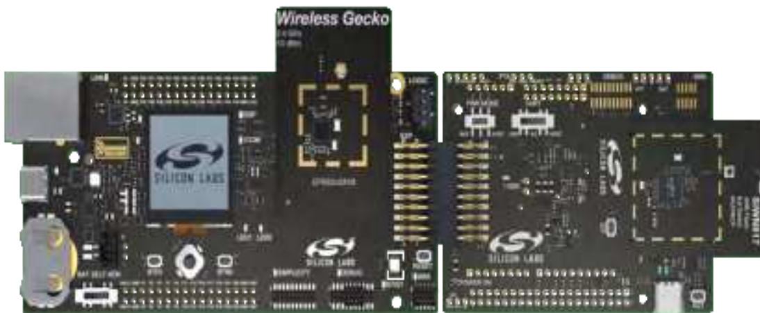
Figure 1.1. Adapter Board (BRD8045A) Connected to a Silicon Labs Wireless Pro Kit Board
