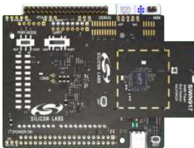
Figure 1.4. Adapter Board (BRD8045C) Connected to a NUCLEO-F411RE
