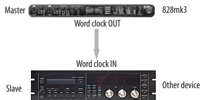
Figure 3-19: Slaving another digital audio device to the 828mk3 via word clock. For the 828mk3 clock source, choose any source besides word clock, as it is not advisable to chain word clock.
