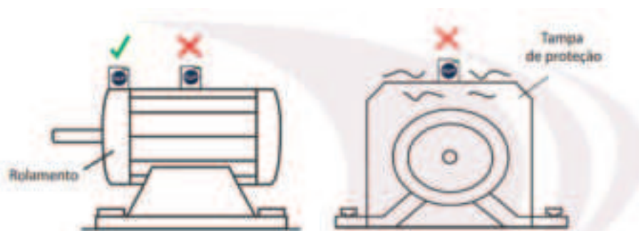
Figure: Installation recommendations
