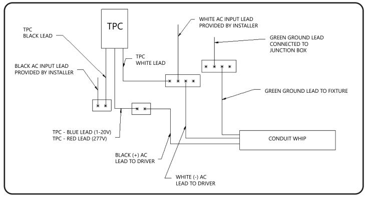
Bring supply leads and ground to the junction box supplied on the Rough in Kit. Be sure to connect leads to existing wire connectors to ensure proper function of thermal protector and fixture.
