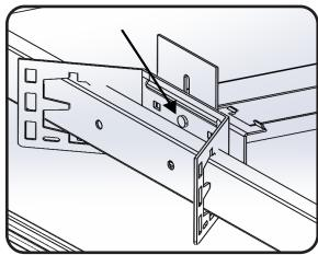
If necessary, the height of the adjustable mounting brackets can be adjusted by loosening the nut so that the bottom of the rough in kit is flush with the top of the ceiling tile.
