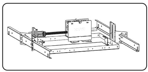
Slide hanger bars through the adjustable mounting brackets on the rough in kit.
