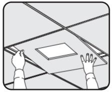
Cut the appropriately sized hole (see table at the right) in the desired ceiling tile. Place the ceiling tile in the ceiling grid.
