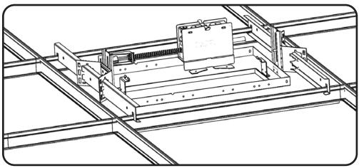
Mount Rough-in-Kit by attaching the hanger bars to the T-Grid ceiling.
