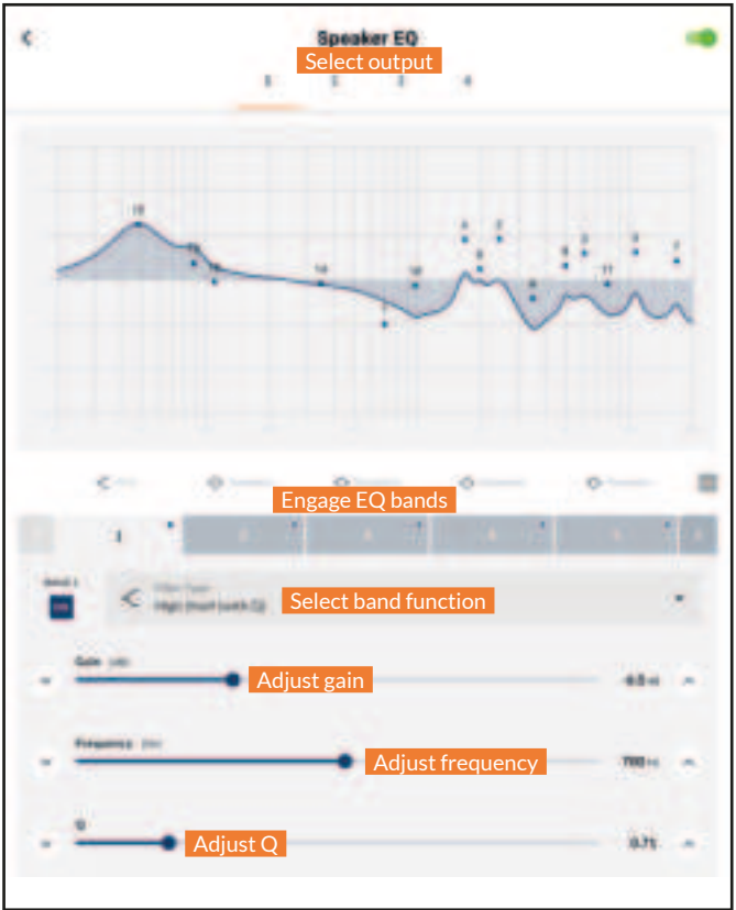
Diagram 6L Speaker Preset parameter adjustment
