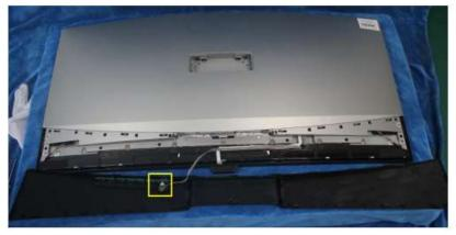
Unscrew the screws to remove the key board from the deco rear cover.
