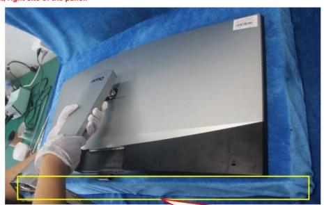
NOTE: The model using the curved surface screen; There must be put soft mat above of
