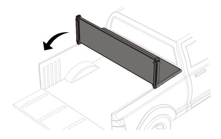
• Open the bungee cord at the front end, fully unfold cover towards the tailgate and ensure cover ailgns on all sides
