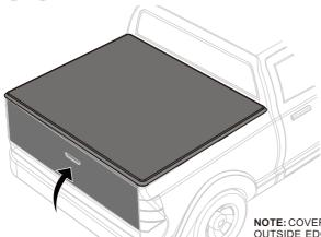
All clamps must be firmly in contact with the lip of the metal bed rail to ensure a firm cover. Finally, close the tailgate to complete the installation.
