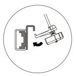
• Attach Front Clamps on to J-shaped aluminum
