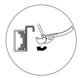
· Attach rear Clamps on to J-shaped aluminum
