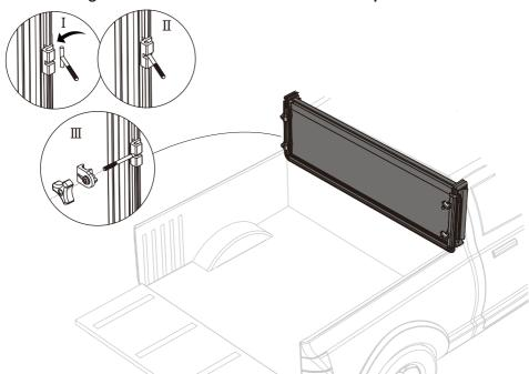
• Slide the front clamp to the best positio, clamp the interface under the metal bed rail, and then use the Triangle screw to rotate into the metal rod to fix the entire clamp
