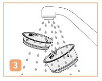
Rinse the front and back of the filter under the faucet, and fina -lly rinse the inner holes and the outer holes with water.
