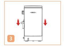
Pour out the remaining water in the water tank. Then set up the water tank vertically and align the buckles to the hole on the back of the machine, and press it down to be parallel to the top of the machine.
