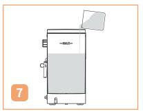
Pour the descaling solution into the water tank.
