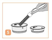
After 5 hours, use a brush to brush the inner surface, inner and outer holes of the filter;
