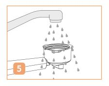
Rinse the inner and outer holes of the portafilter with clean water, and be warned that do not wash the portafilter with any descaler.
