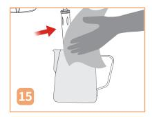
Use a damp cloth to move the position of the steam wand so as to avoid scalding due to the high temperature of the steam wand.
