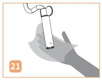
Wipe the outside of the steam wand and the steam wand outlet with a damp cloth to clean the milk stains.
