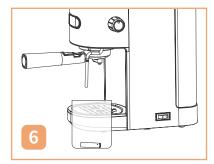
Place the container with that steam wand cover under the steam pipe.
