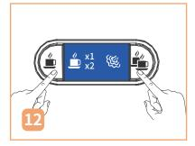
After 5 hours, turn the machine on, long press the double cup and single cup buttons simulta -neously.
