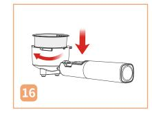
Align the marking dot on the filter with the groove on the portafilter and put it back to the portafilter.
