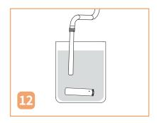
Soak the steam wand cover and steam wand for 5 hours to make sure the limescale is in better contact with the descaling solution and totally dissolved.
