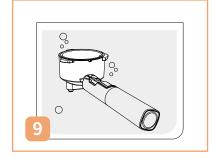
Soak the portafilter in hot water for 10 minutes (do not clean or soak the portafilter in any des -caling solution).
