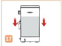
Take out the water tank and fill it with water but do not exceed the MAX marking, and install it onto the machine.
