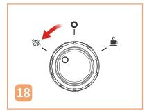
Turn the knob to the Steam icon to release water until all of the water flows out.
