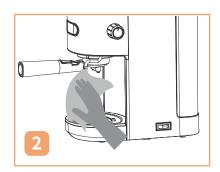
Wrap the steam wand cover with a damp cloth, remove it and put it aside.
