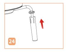
Put the steam wand cover back onto the steam wand.
