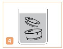
Soak the filter in the remaining descaling solution for 5 hours.
