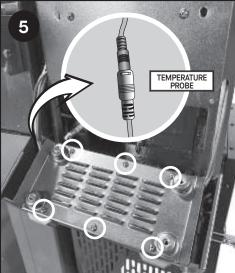
Remove the 6 screws on the back of the controller and remove the rear plate.
