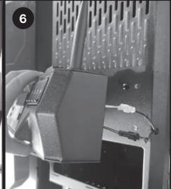
Disconnect two black and white wire connections on the side of the controller.
