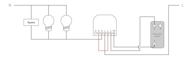
Inclusion of bypass if the LED power output is below 20W.
