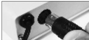
1. Plug the round transformer power cord connector into the back of the scaler, with the arrow on the plug on top.
