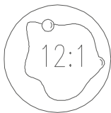
12:1 Gas-liquid Ratio Dense Foam
