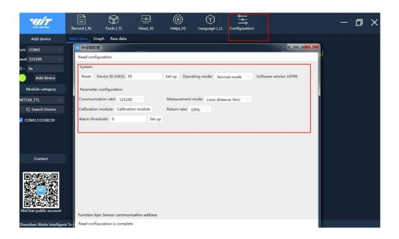
Click "Alarm threshold" after entering the threshold for Alarm Threshold. The alarm threshold setting range is  $40\sim400$ cm (15.748" $\sim157.480$ "). As shown below, set it to 1m (39.370"):
