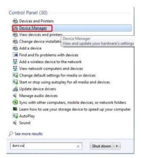
2) After opening the device manager, you will need to open the **Ports (COM & LPT)** tree. The CH340 should show up as **USB-SERIAL CH340 (COM##)**. Depending on your computer, the COM port may show up as a different number.
