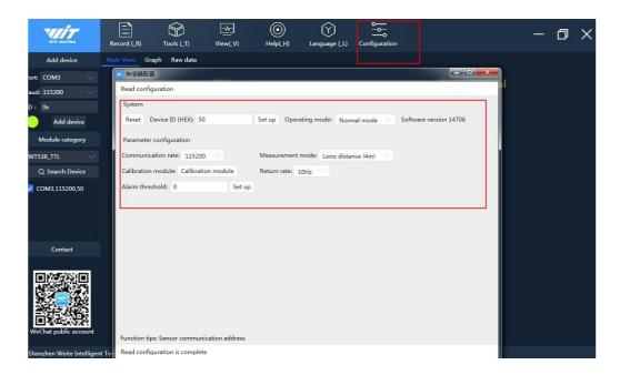
Fix the sensor and calibration object, click "Calibration module".
