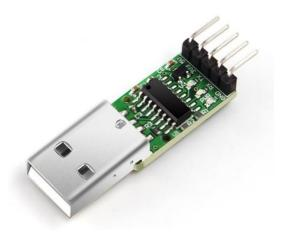
1. USB-TTL serial module (Figure 1): Connect the module to the USB-TTL, then plug it into the computer.
