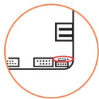
Figure 2-1 Clear CMOS jumper
