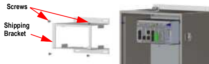
Figure 2-9. Remove Shipping Bracket
