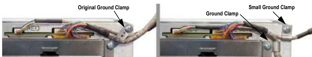
Figure 2-19. Controller Box Shield Grounding
