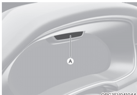
[A] : Interior view camera
