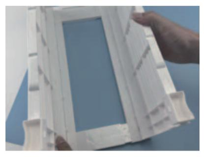
Insert the right side plate into the front and back strips.
