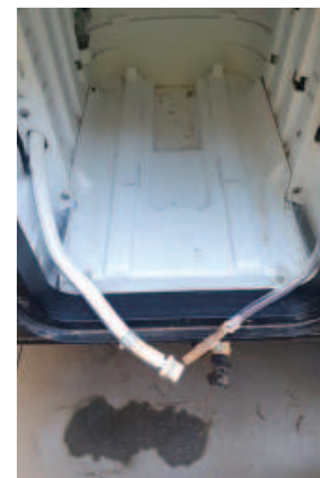
5 Remove the overflow pipe
