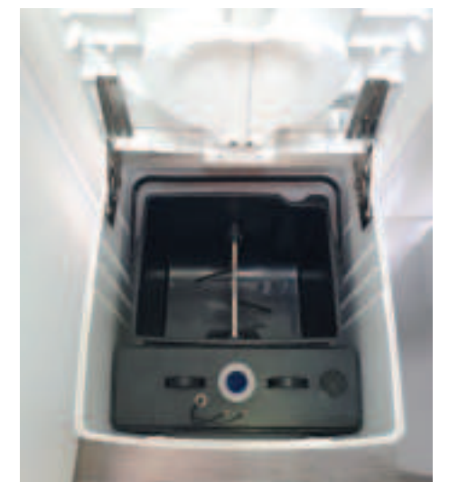
19 Reinsert the containers — add compost medium to the solids container as per the instructions before use
