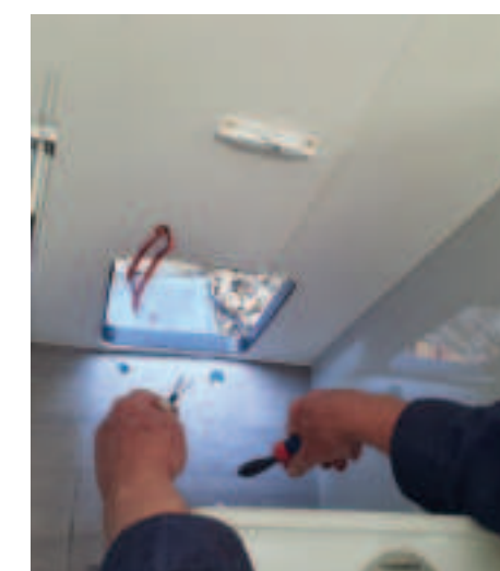
9 Disconnect the 12V power supply
