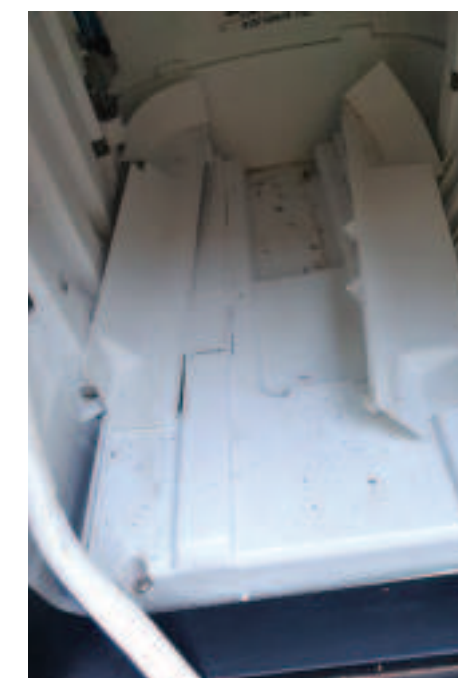
6 Unclip the cassette rails and remove the screws in floor
