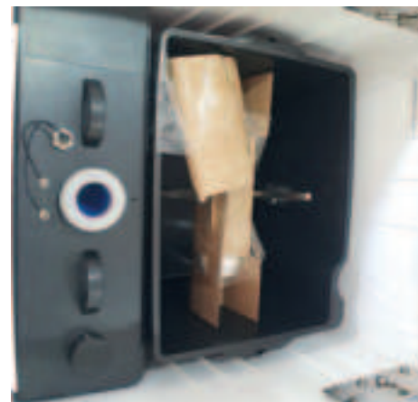
12 Remove the solid and liquid canisters from Cuddy
