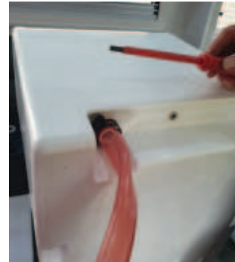
14 Fit vent hose to bottom of unit
