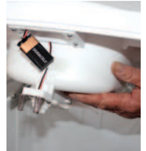
16 Connect 9V battery for liquids container indicator light
