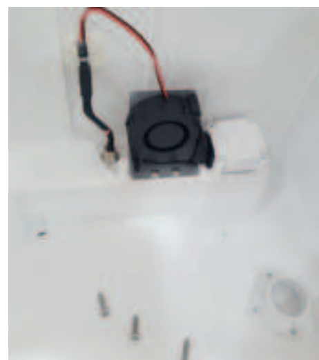
13 Turn the filter base over to vent the 12V fan to outside
