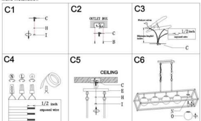
Step C1: Unscrew hex nut (H) and cap nut (I) from single bar (C).
